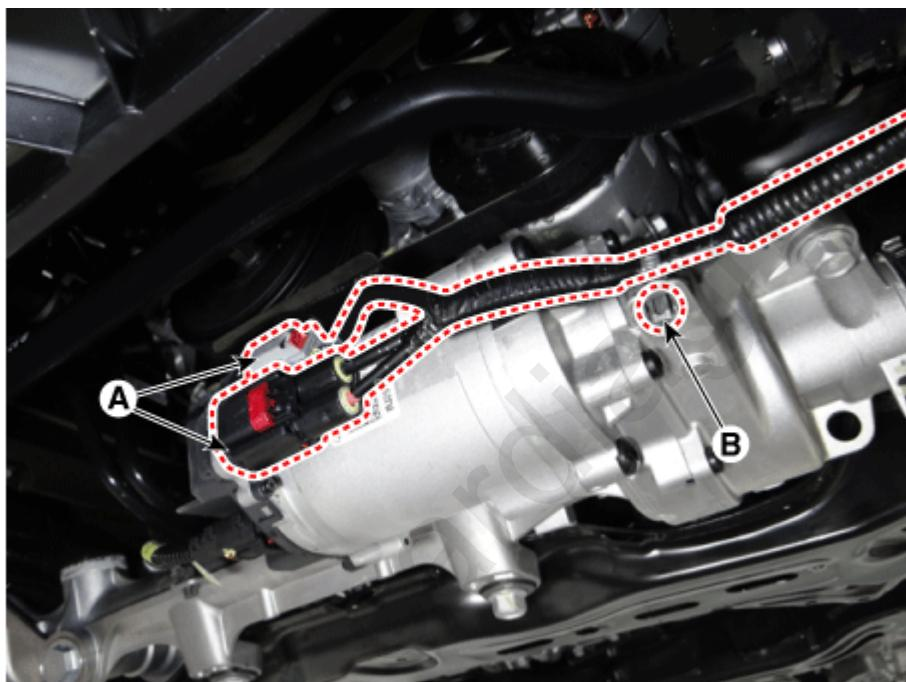
4. Disconnect the R-MDPS wiring clip (A) from the sub frame.
